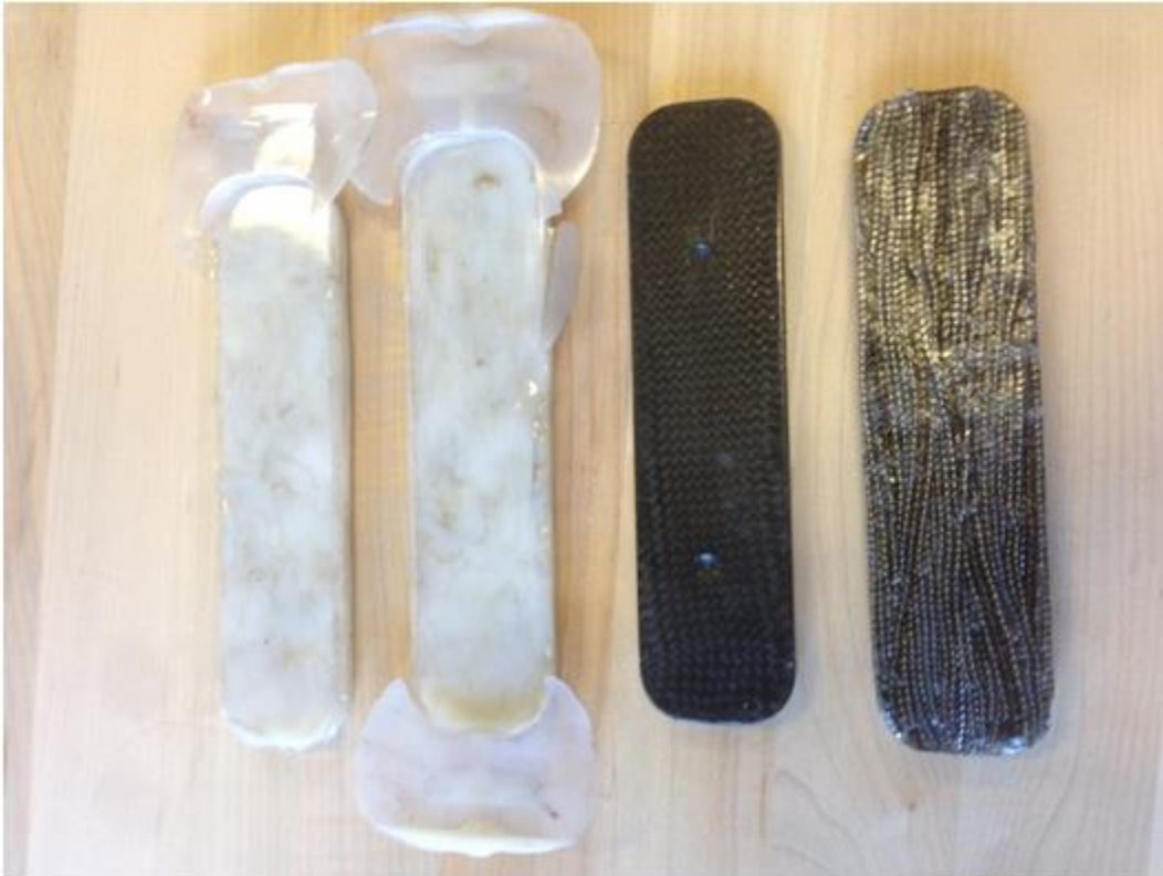
Figure 3.34 -left to right: Recycled High Density Polyethylene (HDPE), (HDPE), Recycled Carbon Fiber and Epoxy resin composite, Lathe turnings and epoxy resin composite
